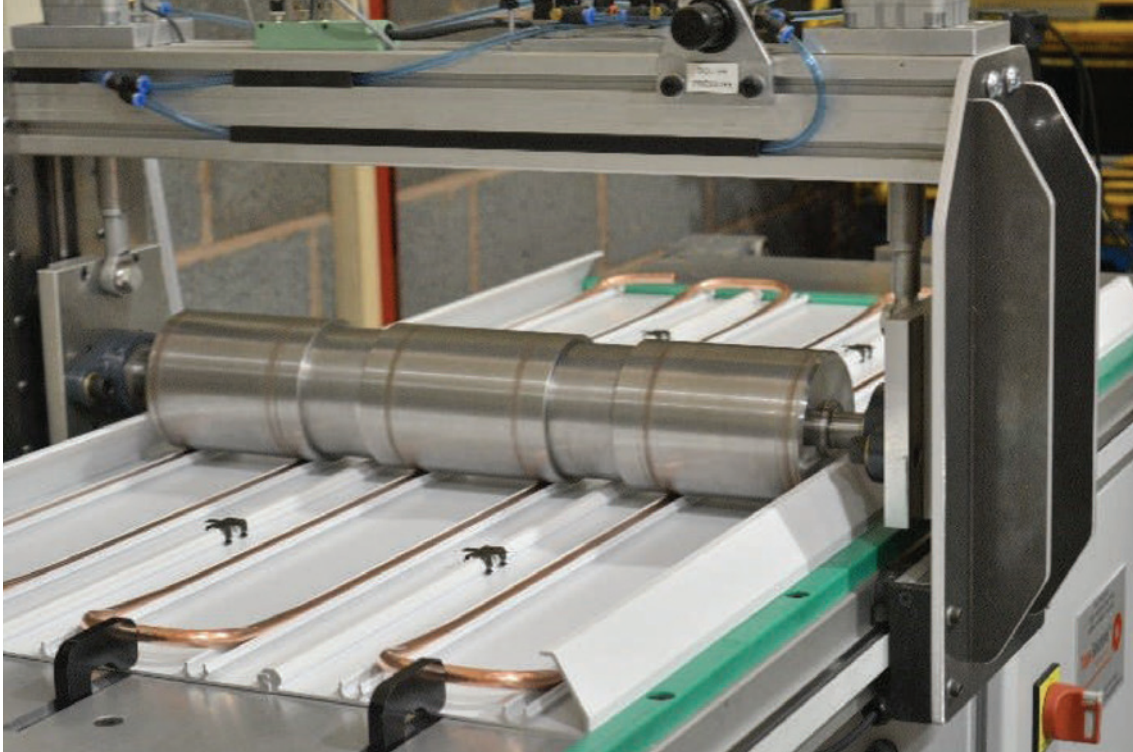
Copper pressed and reshaped into oval pipe carrier.
